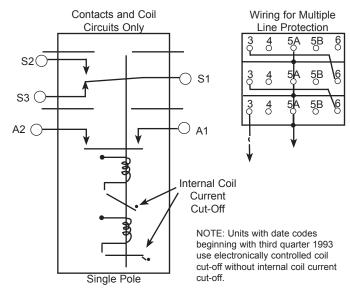
NOTE: Terminals 5A and 5B internally grounded to the mounting leg (s). Integrated wire termination (IWT) module accepts pin contacts P/N M39029/1-100 or -101. Use with insertion/extraction tool M81969/14-02.
