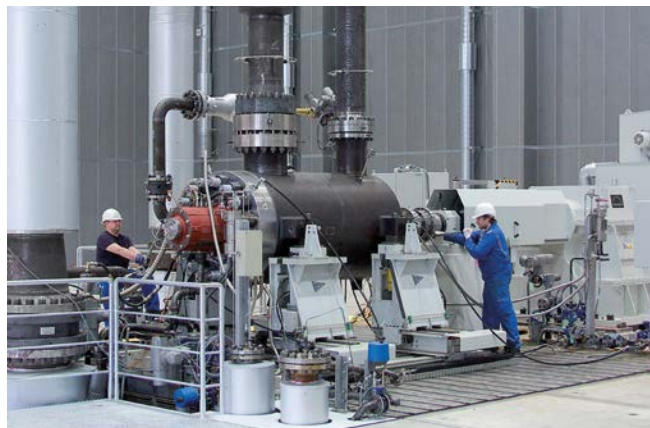
At the world's most modern and efficient test bay for boiler feed pumps, a TUA-800 RENK gear unit ensures reliable power transmission.
