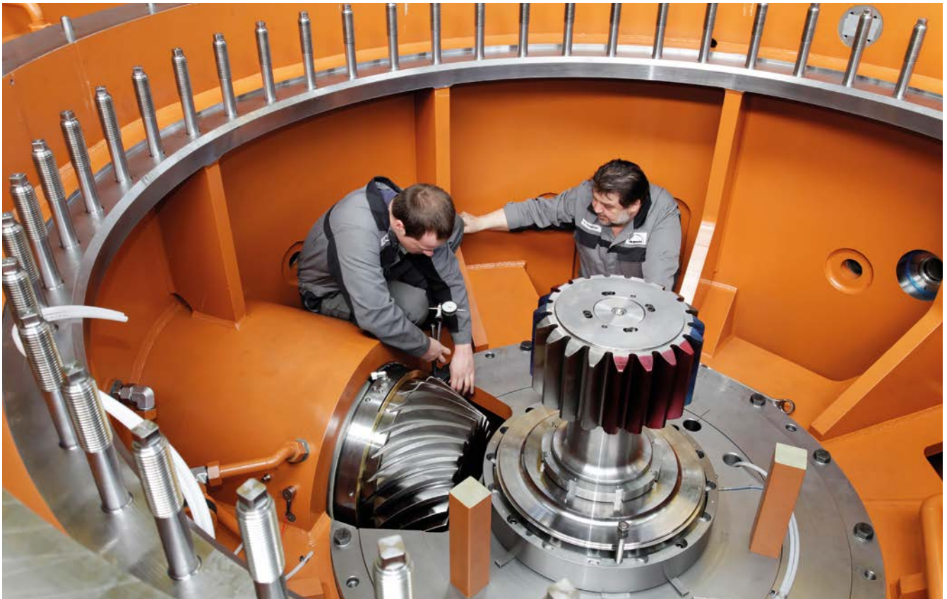
Assembly of a KPBV cement mill gear unit.
