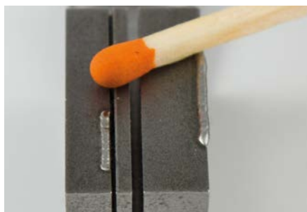
Welding seam build-up - steel material
