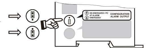
If the jumper is not inserted – or if it is incorrectly inserted – an error message appears when the controller is switched on (\$\sigma\$ section 10.17 "Error messages" on page 37).
