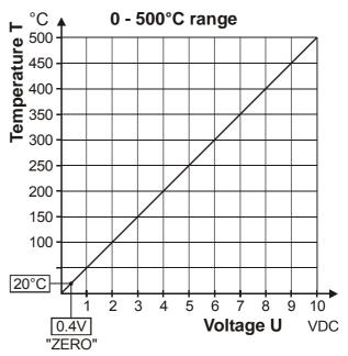
An indicating instrument can be connected to this output in order to visualize the temperature of the heatsealing band.
