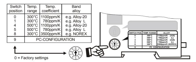
The setting of the rotary coding switch for the temperature range and alloy can be overwritten with the parameter data (\$\\$\\$\ section 10.7\]
