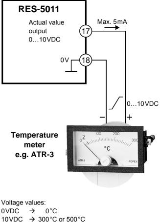
DC → 300°C or 500°C (depending on the controller configuration).
