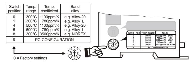
The setting of the rotary coding switch for the temperature range and alloy can be overwritten with the parameter data (& section 10.7 "Parameter object (class: 0x0F)" on page 28).
