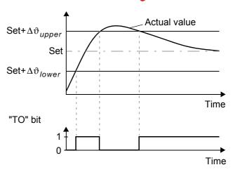
Unlike the "Temperature reached" status bit ("TE" bit), the actual temperature is evaluated independently of the control mode.
