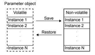
When the controller is switched on, the last values saved in the non-volatile parameter object are automatically restored.
