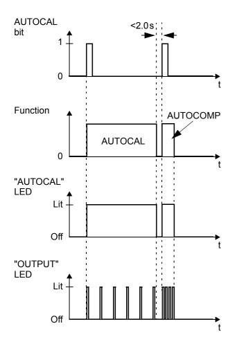
The "OUTPUT" LED blinks repeatedly when the "AUTOCOMP" function is executed and the actual value output (terminals 17+14) is set to 0...3°C (i.e. approx. 0VDC).
