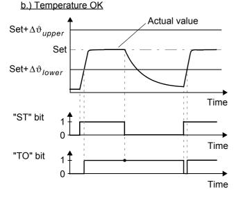
The limits of the tolerance band are adjustable up to a maximum of +-99 K.
