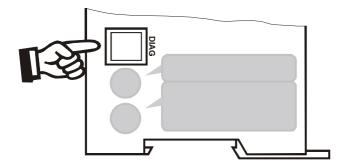
Only a ROPEX communication interface is allowed to be connected to the diagnostic interface. Connecting another device (e.g. a telephone cable) could result in malfunctions or damage to the controller.
