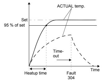
The "heatup timeout" function must be activated by means of the parameter data ( $\$  section 10.7 "Parameter object (class: 0x0F)" on page 28) (default setting: Heatup timeout off).
