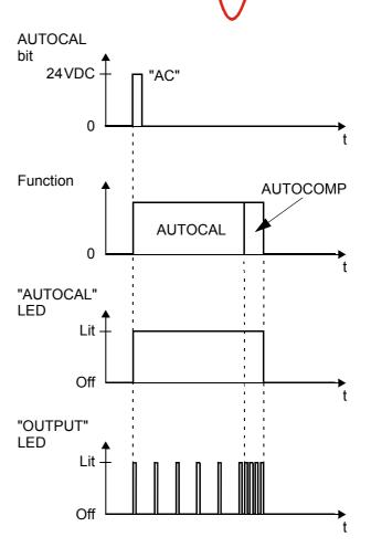
The "OUTPUT" LED blinks repeatedly when the "AUTOCOMP" function is executed and the actual value output (terminals 17+14) is set to 0...3°C (i.e. approx. 0VDC).
