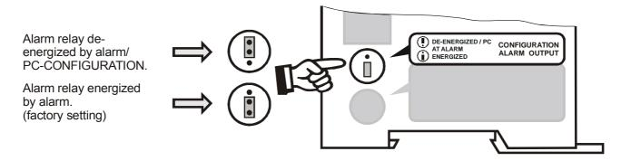
If the jumper is not inserted – or if it is incorrectly inserted – an error message appears when the controller is switched on ( $\clubsuit$  section 10.17 "Error messages" on page 41). If the "Fault relay de-energized at alarm / PC CONFIG-URATION" position is selected, the behavior of the alarm output can be configured in more detail by means of the ROPEX visualization software (∜ see section 10.11 "Diagnostic interface / visualization software" on page 39).
