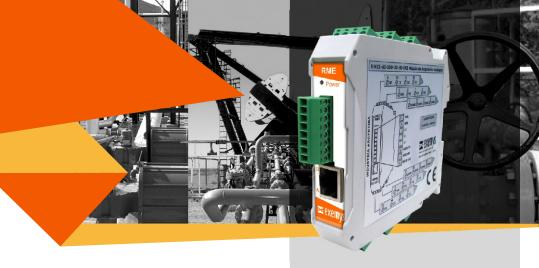
With RME1-PT, you can acquire temperatures from PT100 sensor. This variables can be read in five different ways simultaneously (Modbus TCP, Web Page HTTP, SNMP, CSV and XML).
