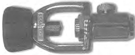
HP Yoke 4000psi service, NOT for use with HP oxygen. Standard scuba yoke with bleeder screw, 1/4" fpt out. Part #: SA4302
