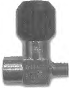
Line Valve 3000psi service, NOT for use with HP oxygen. 1/4" fpt in x 1/4" mpt out. Part #: YVA-3010
