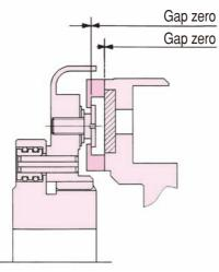
Figure 3: The status of Auto-gap adjustment
