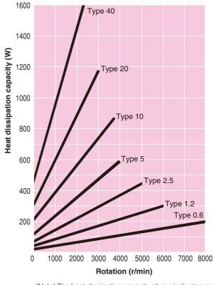
(Note) The heat dissipation capacity above indicates one of each discrete product. For clutch/brake unit products, regard 60% of the heat dissipation capacity in this graph as a standard.
