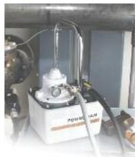
The PA17 used with a flange spreader
