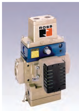
Dual Solenoid Valve No. 303 A most important aspect of double valve design is the incorporation of two separate 3/2 normally closed valve elements which are interconnected within a common valve body assembly. Each of the two valve elements is operated by its own 3/2 normally closed solenoid pilot valve. When simultaneously energized, both main valve elements are operated simultaneously. The probability of both valve elements malfunctioning on the same cycle is
