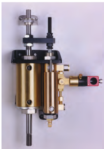
Automatic Ram Control Cylinder No. 305 (Press Brake Applications) Provides a slow speed feature on mechanically actuated, friction clutch press brakes allowing the operator to automatically slow-form a part preventing damage and potential injury due to part "whipping up" during the forming. When used, the ram advances to a predetermined position above the work with the clutch fully engaged (fast down). At this point, the ram will stop allowing for realignment of the part before forming. The foot switch is then actuated a second time and the ram will advance slowly forming the part and then return to the top of the stroke at a high speed (fast return). The Ram Control can be adjusted to provide the best speed for the part being formed.
