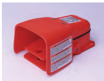
Electric Foot Pedal No. 302 An oil-tight foot switch. Contains one set, normally-open contacts, and one set normally-closed contacts. Includes a treadle guard to protect against accidental tripping. "Requires a point of operation guard when used for machine actuation," such as safety light curtains or safety interlock systems.
