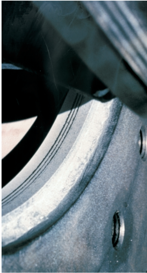
Dye Test showing no wear or rubbing
