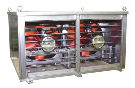
They are mainly used as brake resistor on top of cranes in harprotect the inside of the resistor unit when not in operation. bors. Two or four high power ventilators provide a strong air flow that cools a number of steel tube elements.
