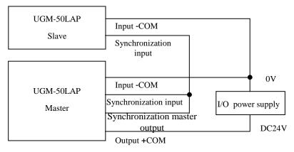
As shown in the figure above, it is possible to synchronize the motor rotation of the slave with the motor rotation of the master according with shifted the scanning time of each slave sensor by setting phases of each slave sensor.
