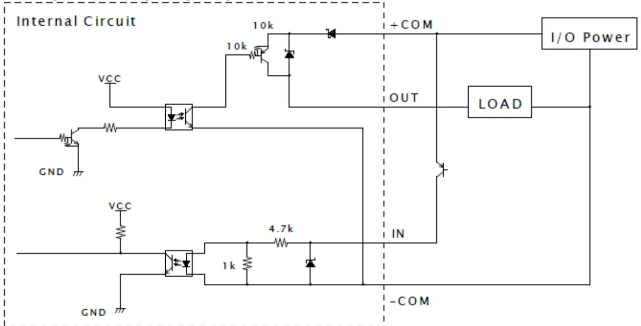
Connect both +COM and -COM to I/O Power.
