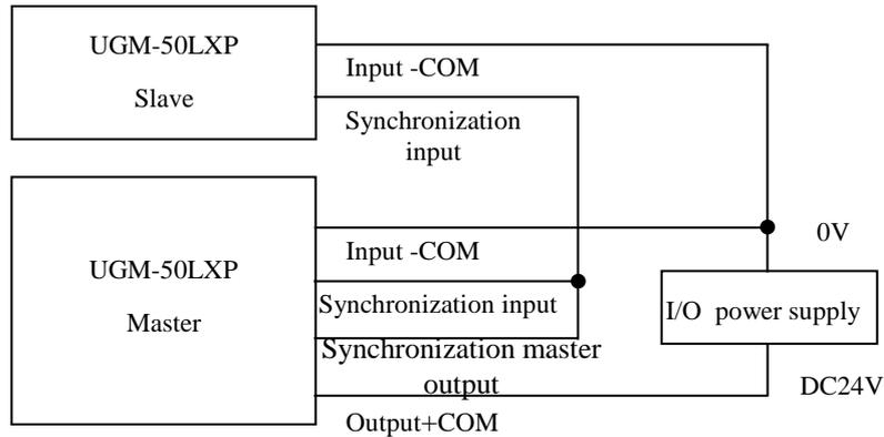
As shown in the figure above, it is possible to synchronize the motor rotation of the slave with the motor rotation of the master according with shifted the scanning time of each slave sensor by setting phases of each slave sensor.
