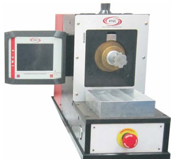
Linear ultrasonic metal welder with 4'000 N clamping force and max. 6'500 W output power
