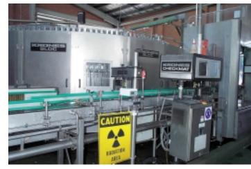
A bottle and can filling line is integrated with a UNIMETER XQL connected to a magneto transducer. From the digital reading, the bottle or can height is determined. This value is then used to set the height of the filling nozzle in the line. The UNIMETER XQL has two set points.
