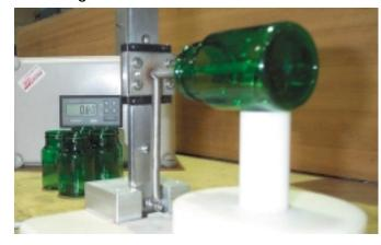
A producer of natural health products uses UNIMETER XQLs to measure and monitor both mould temperature and bottle thickness in the production of their bottles and containers. This provides an accurate and easy to operate measurement system. The UNIMETER XQL's USER OFFSET and TARE functions allow for quick and easy calibration.
