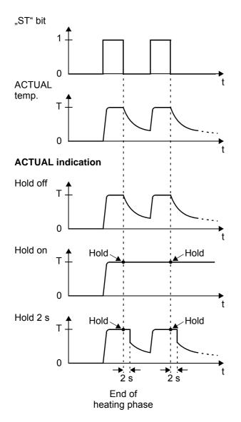
The "hold mode" function must be activated by means of the PROFINET parameter data (\$ section 9.7 "Parameter data" on page 29). (Default setting: Hold mode off)
