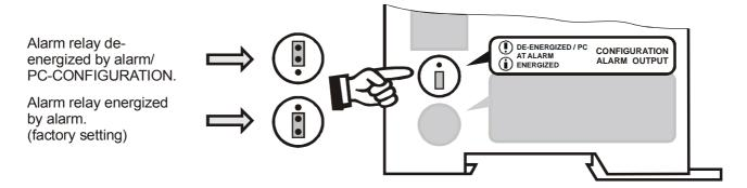
If the jumper is not inserted – or if it is incorrectly inserted – an error message appears when the controller is switched on ( $\clubsuit$  section 9.17 "Error messages" on page 37). If the "Fault relay de-energized at alarm / PC CONFIG-URATION" position is selected, the behavior of the alarm output can be configured in more detail by means of the ROPEX visualization software (∜ see section 9.11 "Diagnostic interface / visualization software" on page 34).
