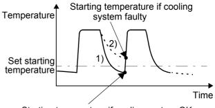
Starting temperature if cooling system OK
