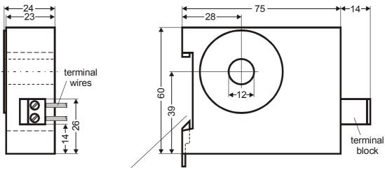
Snap-on for DIN-rail 35 x 7,5mm or 35 x 15mm (DIN EN 50022)
