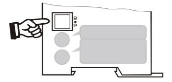
Only a ROPEX communication interface is allowed to be connected to the diagnostic interface. Connecting another device (e.g. a telephone cable) could result in malfunctions or damage to the controller.
