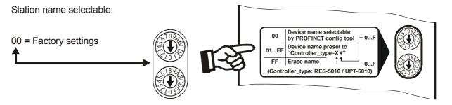
By assigning station names using rotary coding switches, it is possible to replace a device in an existing machine without a programming tool. The replacement device must simply be configured with the same switch settings.
