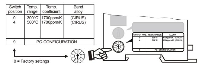
The setting of the rotary coding switch for the temperature range and alloy can be overwritten with the parameter data ( section 9.7 "Parameter data" on page 29).
