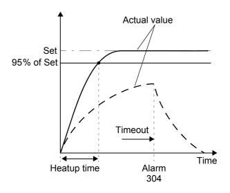
The "Heatup timeout" function must be activated by means of the PROFINET parameter data (% section 9.7 "Parameter data" on page 29). (default setting: Heatup timeout off)
