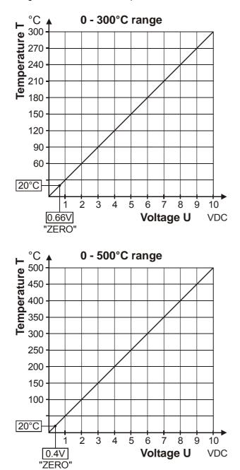
An indicating instrument can be connected to this output in order to visualize the temperature of the heating element.
