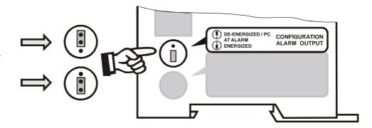
If the "Fault relay de-energized at alarm / PC CONFIG-URATION" position is selected, the behavior of the alarm output can be configured in more detail by means of the ROPEX visualization software (\$\sigma\$ see section 9.11 "Diagnostic interface / visualization software" on page 37).
