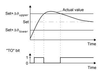
Unlike the "Temperature reached" status bit ("TE" bit), the actual temperature is evaluated independently of the control mode.
