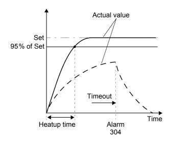
The "Heatup timeout" function must be activated by means of the EtherNet/IP parameter data (\$\infty\$ section 9.7 "Parameter object (class: 0x0F)" on page 27).
