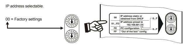
The "01...FE" switch positions allow an IP address to be assigned, or the DHCP client switched on and off, via the EtherNet/IP interface either using a software tool (e.g. Rockwell's "BOOTP / DHCP Server") or by manually accessing the TCP/IP object. These settings
