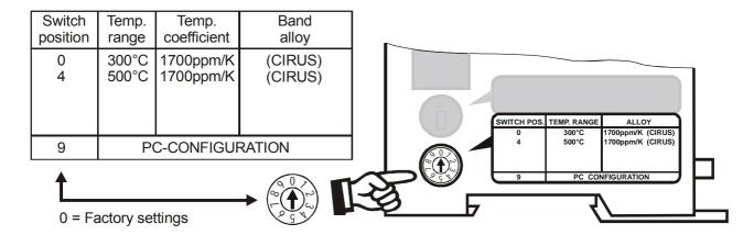
The setting of the rotary coding switch for the temperature range and alloy can be overwritten with the parameter data (\$\infty\$ section 9.7 "Parameter object (class: 0x0F)" on page 27).
