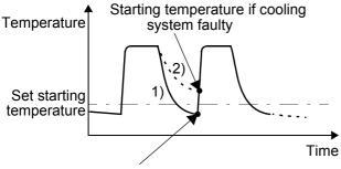
Starting temperature if cooling system OK
