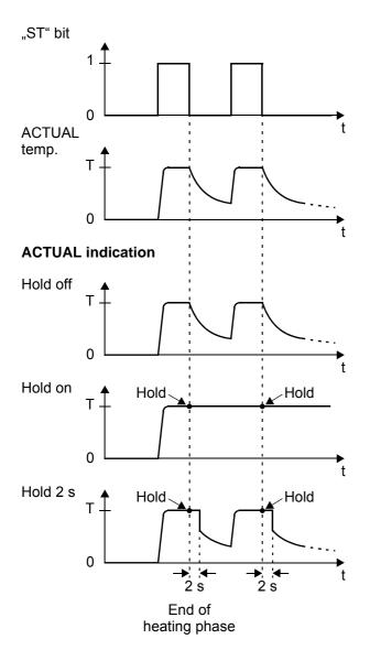
The "hold mode" function must be activated by means of the EtherNet/IP parameter data (\$ section 9.7 "Parameter object (class: 0x0F)" on page 27).
