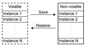
When the controller is switched on, the last values saved in the non-volatile parameter object are automatically restored.
