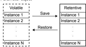
When the controller is switched on, the last values saved in the retentive parameter object are automatically restored.
