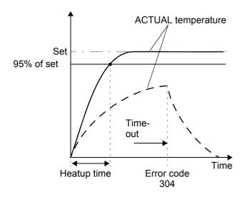
The "Heatup timeout" function must be enabled for use in the parameter data (♥ section 6.7 "Parameter object (class: 0x0F)" on page 23) (default setting: heatup timeout off).
