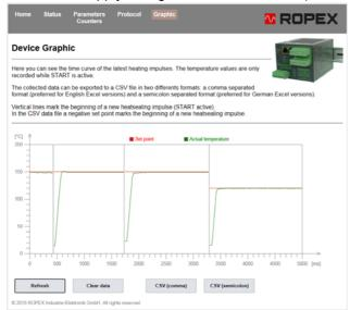
The vertical lines mark the beginning of a new heatsealing impulse ("ST" bit set). A negative set point indicates the start of a new impulse in the exported data. Cooling processes are not normally visible because they take place when the "ST" bit is reset.
