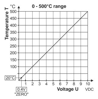
An indicating instrument can be connected to this output in order to visualize the temperature of the heating element.
