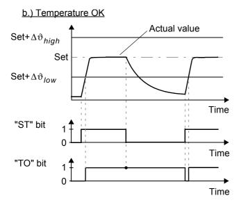
The limits of the tolerance band are adjustable up to a maximum of  $\pm 99$  K.
