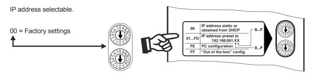
The "01...FE" switch positions allow an IP address to be assigned, or the DHCP client switched on and off, via the EtherNet/IP<sup>TM</sup> interface either using a software tool (e.g. Rockwell's "BOOT / P-DHCP Server") or by manually accessing the TCP / IP object. These settings
