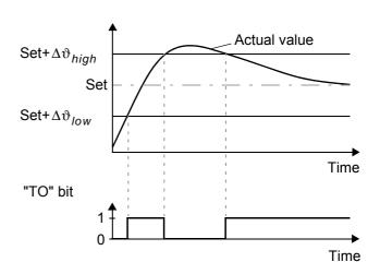
Unlike the "Temperature achieved" status bit ("TE" bit), the actual temperature is evaluated independently of the control mode.
