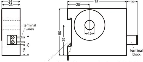
Snap-on for DIN-rail 35 x 7,5mm or 35 x 15mm (DIN EN 50022)
