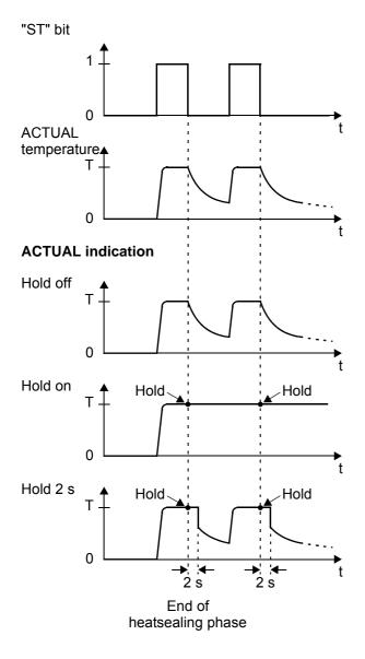
The "Hold mode" function must be activated in the parameter data (♥ section 6.7 "Parameter object (class: 0x0F)" on page 23) (default setting: hold mode off).
