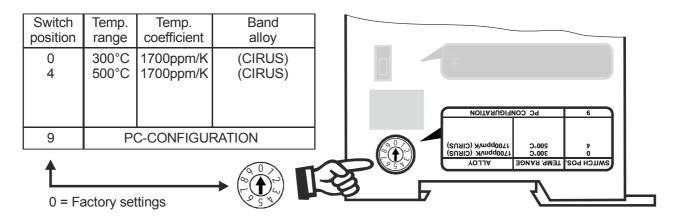
The setting of the rotary coding switch for the temperature range and alloy can be overwritten with the parameter data (\$\infty\$ section 6.7 "Parameter object (class: 0x0F)" on page 23).
