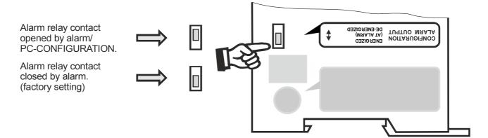
If the switch is set to "Alarm relay de-energized at alarm / PC CONFIGURATION", you can select more alarm output configurations in the ROPEX visualization
