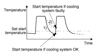
If the cooling system is intact, curve 1) applies. If the cooling system is faulty, curve 2) applies instead
