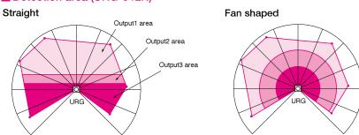
Notre) This device shows the detection area on the basis of the center position of scanning.
