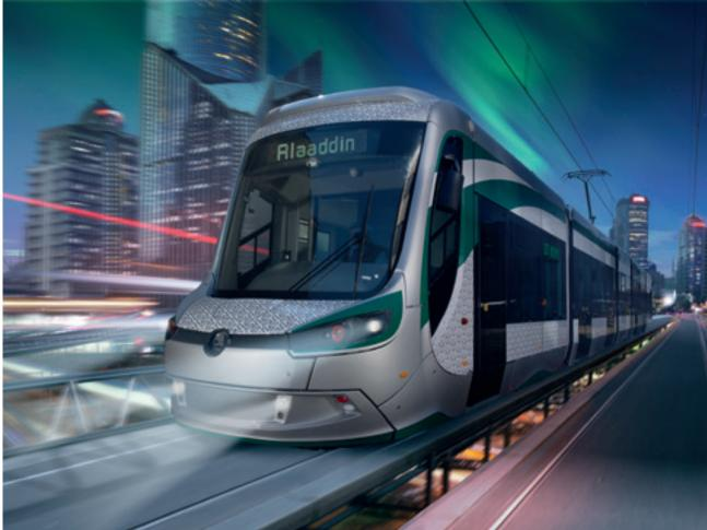
The ForCity trams are divided into four basic types. The first type is the ForCity Alfa with a completely pivoting bogie and gearless design. These vehicles are particularly suitable for tracks with less than ideal operating conditions. The second type of vehicle is the modernised ForCity Alfa tram. This range is accompanied by the ForCity Classic that uses a non-pivoting bogie and which is especially designed for straighter, modern tracks.
