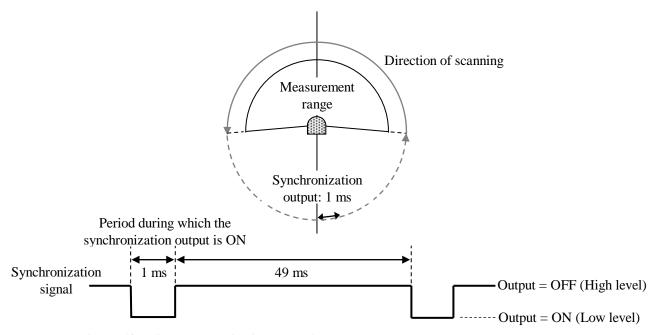
During malfunction, synchronization output is OFF.
