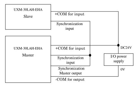
Synchronization output of the master sensor is connected to the synchronization input of the master itself and to the synchronization input of all slave sensors.
