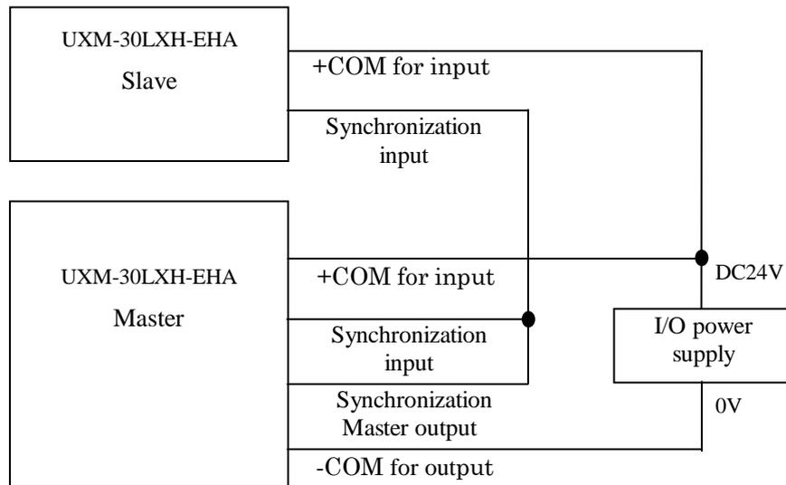
Synchronization master output of the master's sensor is connected to the synchronization input of the master itself and to the synchronization input of all slave sensors.
