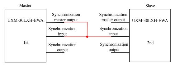
Synchronization master output of the master's sensor is connected to the synchronization input of the master itself and to the synchronization input of all slave sensors.
