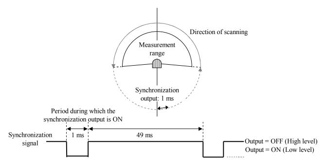
During malfunction, synchronization output is OFF.
