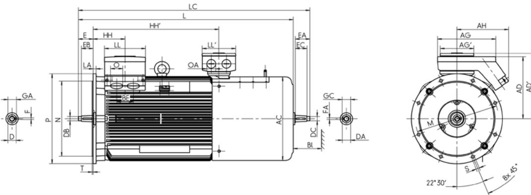
**Three-phase motors with slip-ring rotor
