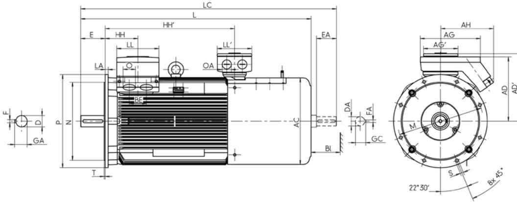
**Type of construction IM B5K [IM 3003], IM 3004; up to size 200, IM V1K [IM 3013], IM 3014**
