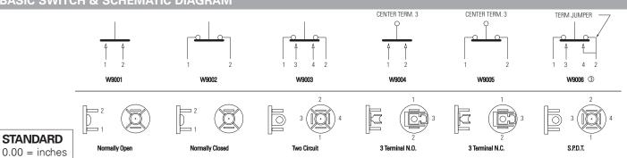
3 For W9006 or SPDT circuit, mount terminal jumper to terminals #2 and #4.
