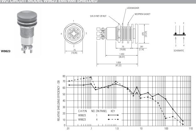
Graphic illustration defines relative shielding efficiency of RFI shielded component/ components over
