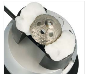
Mould jaws made of modelling granulate
