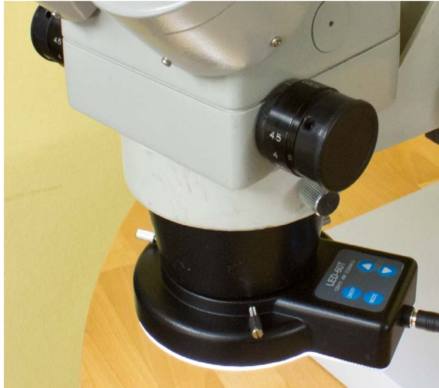
Use of the LED ring light with segmental switching on the SM-200 stereomicroscope.
