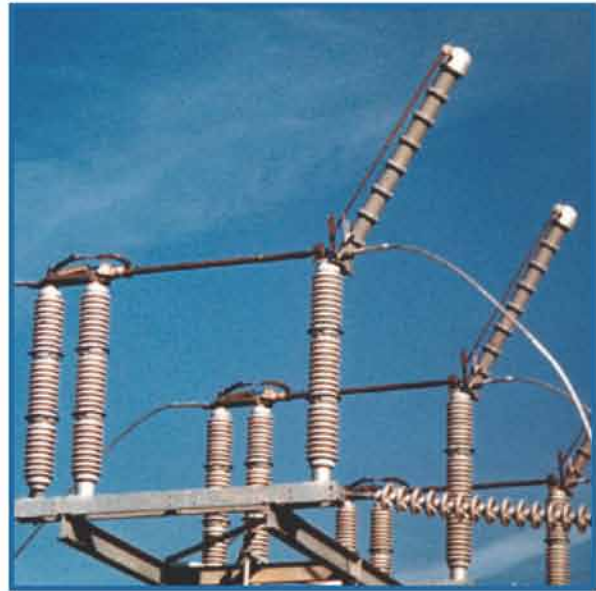
138kV typical full load-break switch combining the Series JMVI Interrupter with the Joslyn Hi-Voltage® Series RF-2 Vertical-Break Switch. The Series JMVI Interrupter converts the isolating switch for full load switching at system voltages up to 230kV.
