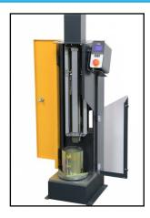
subsequent blows, granting a precise and uniform blows distribution. The rotating base has screw clamping system for the moulds locking.
