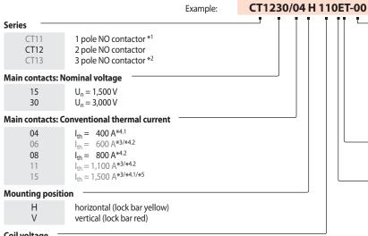
**Auxiliary contacts** 1x S870\*6.2 (a1) 1x S870\*6.2 (b<sub>0</sub>) M3 screw-type terminals 00 2x S826\*6.1/\*6.3 1x S870\*6.2 (a1) M3 screw-type terminals 1x S870\*6.2 (b<sub>0</sub>) 01 2x S826\*6.3 Flat tabs 6.3 x 0.8 4x S826\*6.3 M3 screw-type terminals 02 4x S826\*6.3 Flat tabs 6.3 x 0.8 03 Surge suppression/type of coil Suppressor diode / standard coil \*4.3 Double coil controller (DCC) / double coil \*4.4 CM Coil tolerance -30 % ... +25 % Е
