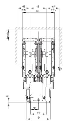
CT1230/08 Dimension diagram double pole NO contactor for 3,000 V / 800 A (standard version)
