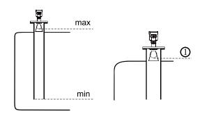
You are advised to opt for installation with standpipe (or bypass tube) to avoid the influence on measurement caused by barriers inside vessels, foam generation.
