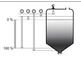
Reference Plane for Measurement: the thread or seal plane of flange Measurement blanking zone: the area between measurement reference plane and the antenna end.
