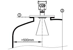
Note: Minimum distance of 500mm between measurement and vessel wall during installation
