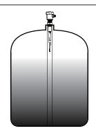
Installation with a plastic standpipe can avoid the generation of multiple false echoes while the measurement being mounted on the center of vessel top. You are advised to use PP or PTFE if the measured medium is strong acidic or alkaline.
