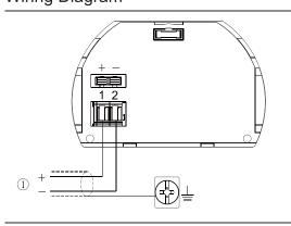
2-wire wiring used for HART
