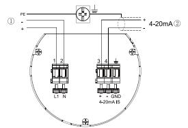
Wiring plan suitable for 4-wire/2-chamber structure
