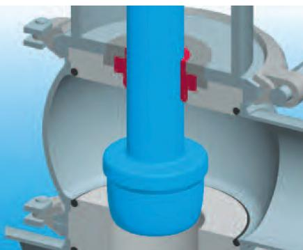
**Stem seal with combination sealing element**
