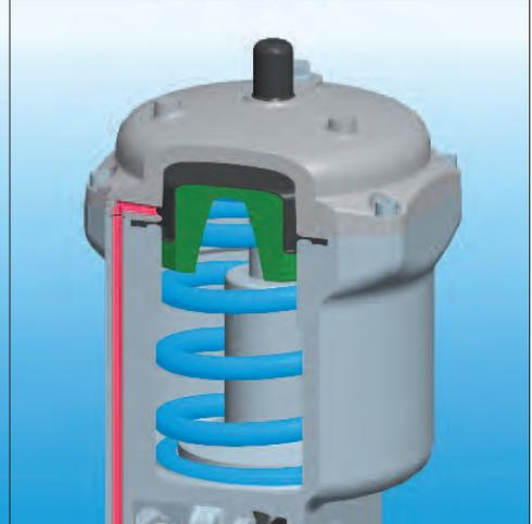
The ARCA-specific diaphragm enclosure and integrated air ducting have been integrated as a design feature. Characteristic for this pneumatic rotary actuator is the rolling diaphragm, which operates very uniformly with hysteresis-free torque output throughout the entire range. An emergency override can also be ordered or retrofitted.
