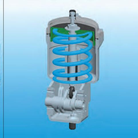
The ARCAtorque 840 targets rotary actuators designed quarter-turn movements. Four sizes are available, each of which has a double-sided connecting flange compliant with DIN/ISO requirements. The «spring to open» and «spring to close» safety functions are easy to realize with this rotary actuator. Instrumentation can be added using the same DIN/ISO connection flange.
