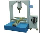
Being a low cost alternative, QCRT-MFXT testing machine combines precision and simplicity with the unique design of the manual power pack. Hand Operated Hydraulic Power Pack enables even an inexperienced operator to perform the flexure tests on-site. The QCRT-MFXT flexural machine have the accuracy of Class 1 starting from 2% of the full capacity.
