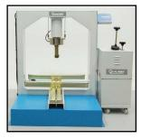
with range of 200 kN capacity flexure testing machines allow inexperienced operators to perform the test. The flexural testing machines consist of heavy duty welded frame, hydraulic power pack with data acquisition system QCRTDAS. The QCRT-SAFXT Concrete Semi-Automatic Flexural Testing Machine have the accuracy of Class 1 starting from 2% of the full capacity. Flexural test assemblies should be ordered separately.
