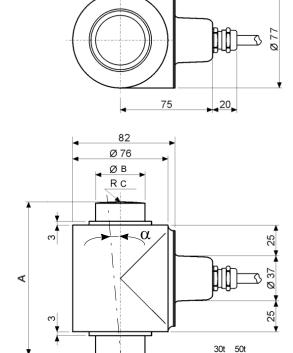
$\alpha$  : Allowed maximum angle of inclination: 5°.
