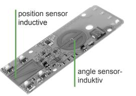
... from µm up to cm inductive or capacitive
