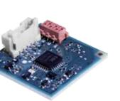
Capacitive measurement fill level sensor for conductive and non-conductive media. With non-conductive media, the electrodes are arranged coaxially. With conductive media a single insulated electrode suffices.
