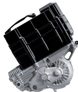
Fully integrated PMS Motor of KTM E-Enduro Freeride E
