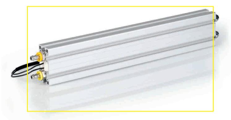
By using water-cooled resistors, the heat development that usually occurs at the location of use is prevented. During braking processes, the electrical drive energy is converted to heat energy. This heat energy is absorbed by the water and can be re-used. Whereas in smaller resistor systems the cooling water is routed directly through the resistor profile, heat exchangers are used in resistors with a power > 50 kW.
