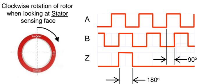
A leads B for clockwise rotation of rotor
