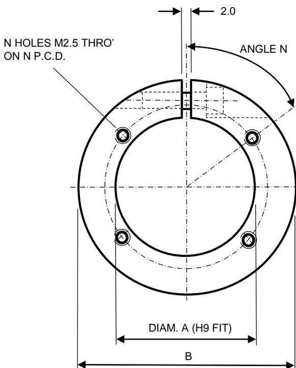
SIDE ELEVATION SHOWING POSITION OF A SCREW MOUNT ROTOR & A STATOR
