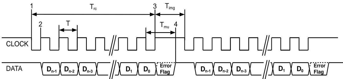
T: Clock Period ( $1/T = 100 \text{ kHz to } 2 \text{ MHz}$ )
