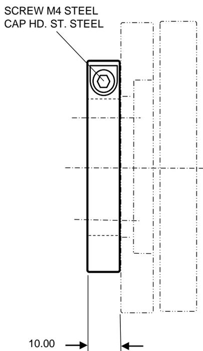
NOTE REGARDING ATTACHMENT METHOD. FIRSTLY, ATTACH CLAMP TO ROTOR USING 'N' SCREWS. TIGHTEN M4 SHAFT CLAMP SCREW TO SECURE TO SHAFT AND ONLY THEN TIGHTEN THE 2 SCREWS ADJACENT TO SHAFT CLAMP SPLIT LINE.
