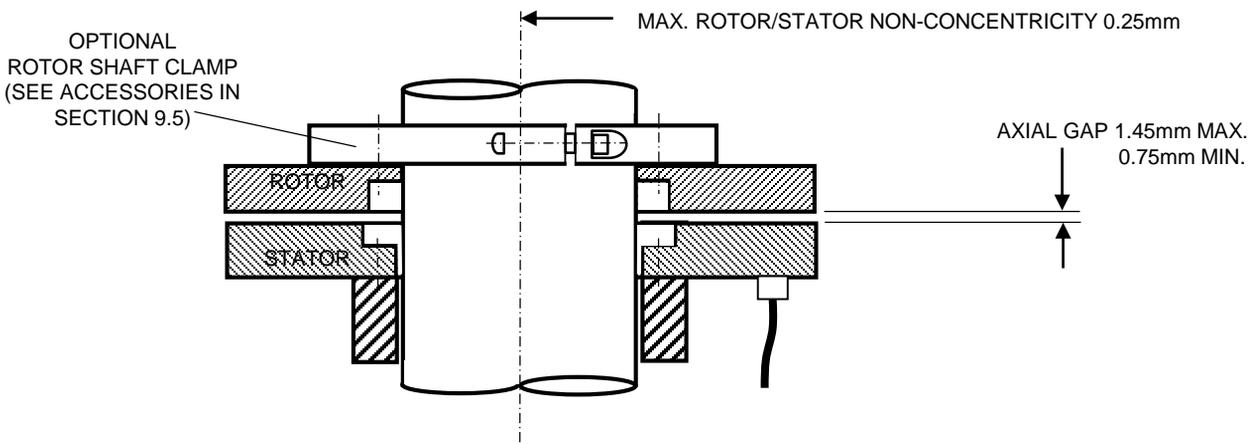
All formats of IncOder can be installed using a circumferential clamp in the host equipment. This applies to Rotor or Stator. Preferably the C-ring's gap is closed by at least one screw.
