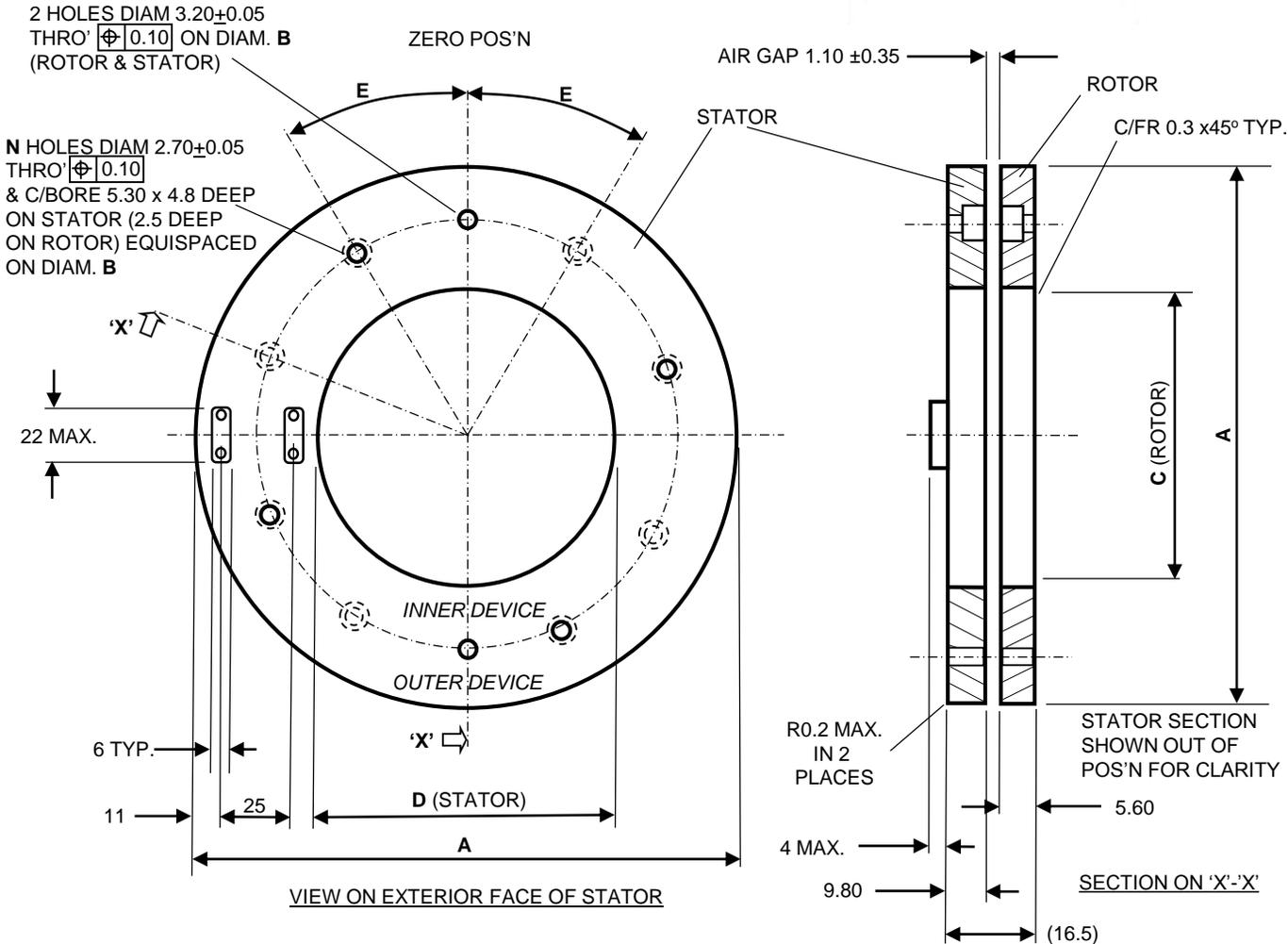
Duplex IncOders are electrically redundant:- 2 electrically independent IncOders in 1 package – the first on the outer annulus, the second on the inner. The range starts at an O.D. of 125mm with axial connections (AC1) or integral flying leads (AFL1-5). Note - measurement performance is quoted for the outer annulus device.
