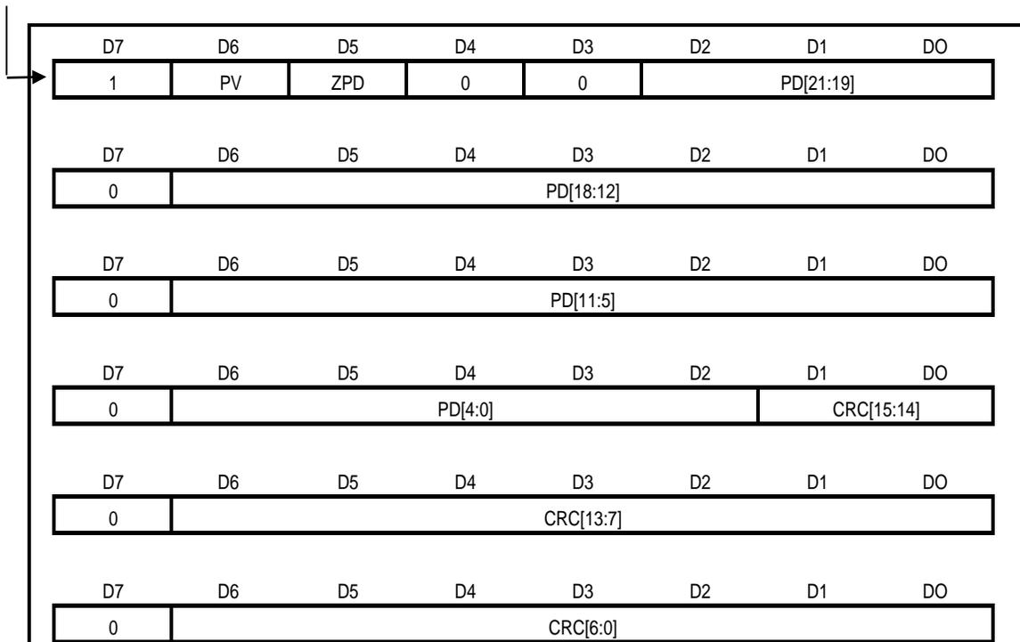
**Data Definition for Asynchronous Serial Interface**
