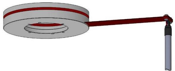
**RFC10** – 2m upward cable & 100mm radial
