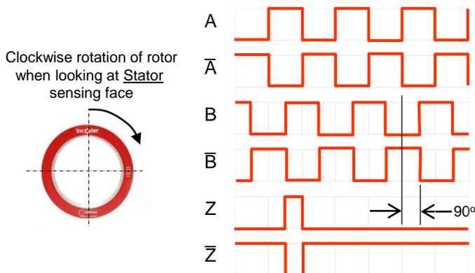
A leads B for clockwise rotation of rotor
