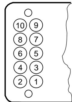
REMOVE THESE SCREWS ONLY IF ABSOLUTELY NECESSARY. IF REMOVED, ENSURE CONNECTIONS ON U/SIDE OF CONNECTOR ARE ALTERNATIVELY PROTECTED FROM CONTACTING CONDUCTIVE OR ABRADING SURFACES.
