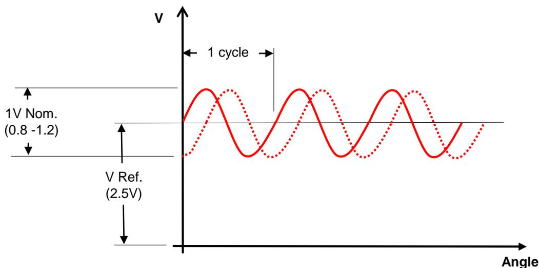
Analogue Voltage Interface versions of IncOder are available for all sizes of IncOder (other than 37, 58 & 300mm) with max. voltage outputs of 4.5, 5.0, 9.5 and 10.0V in 90°, 180°, 270° & 360° spans with either clockwise or counter-clockwise directions. Zero, direction & span are field programmable without a PC. The following sections 6.8.1 - 7 describe the various Product Options and field programming:-
