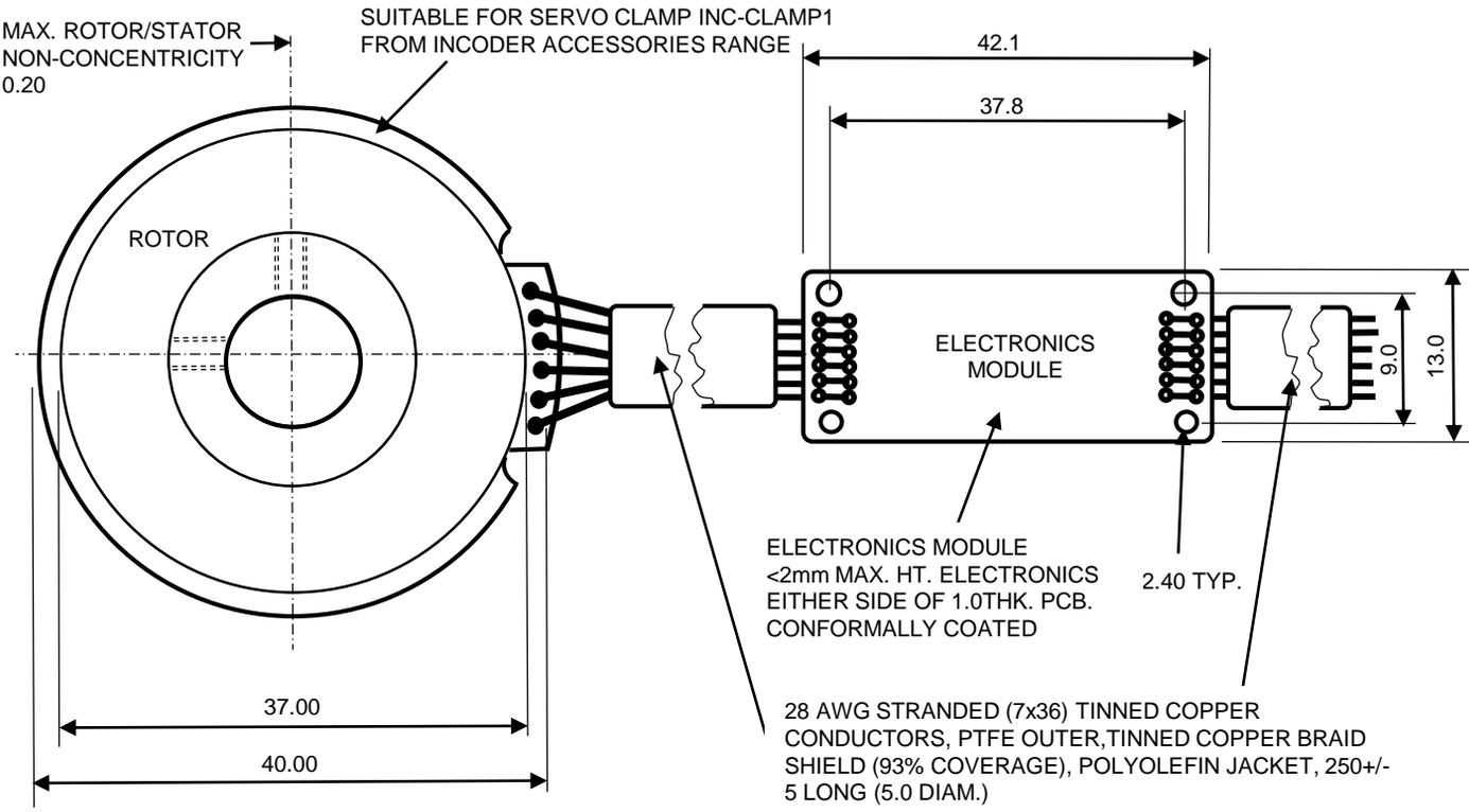
OPTIONS FOR DIM C = 5.00; 6.00; 6.35 AND 8.00 ALL WITH H7 TOLERANCE - SEE SECTION 8 ON HOW TO SELECT BY PART NUMBER.
