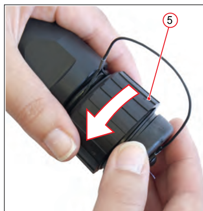
Fig. 30: Screw down union nut hand-tight
