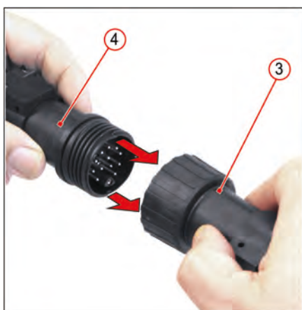
Fig. 28: Slide off plug (3) from receptacle (4)
