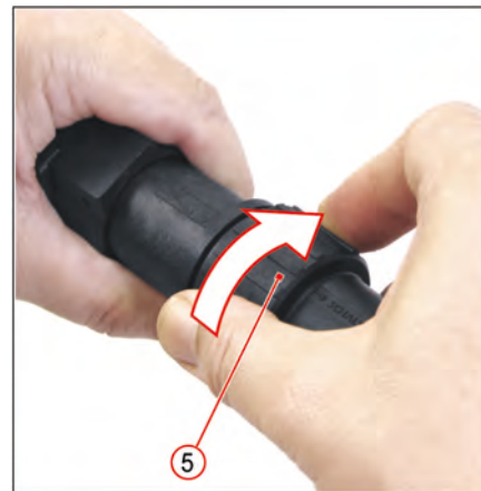
Fig. 26: Screw union nut (5) on thread of receptacle
