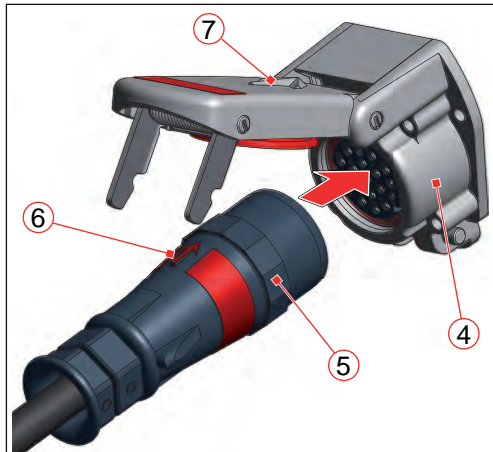
Fig. 21: Align arrow (6) on plug congruent with arrow (7) on the receptacle lid
