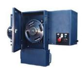
The Charpy Specimen Machine uses a 5 bladed cutter with easily replaceable inserts, used without any cutting lubricants
