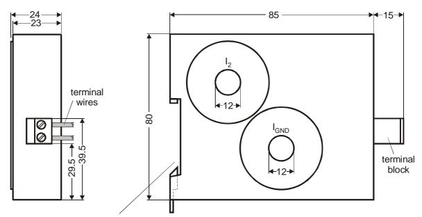
Snap-on for DIN-rail 35 x 7,5mm or 35 x 15mm (DIN EN 50022)
