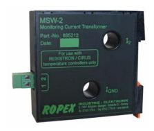
In certain applications with RESISTRON or CIRUS temperature controllers, it is necessary to detect shortcircuits between the heatsealing band and ground or the housing. In this case, the control system must be immediately switched off. The MSW-2 monitoring current transformer can be used for this purpose.
