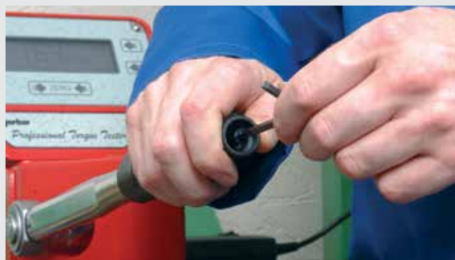
Setting a 'P' Type Torque Wrench
