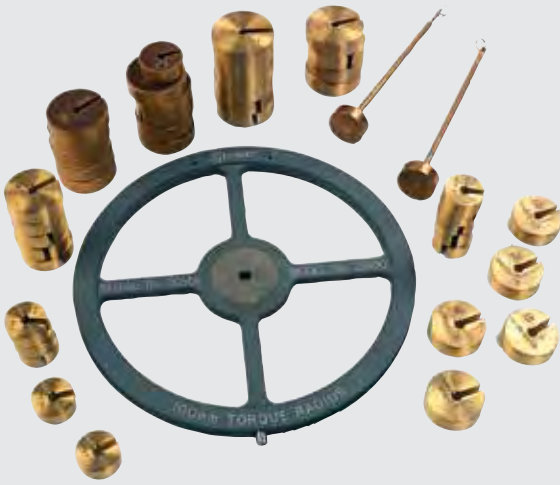
Calibration Disc with weight sets
