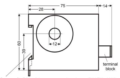
Snap-on for DIN-rail 35 x 7,5mm or 35 x 15mm (DIN EN 50022)
