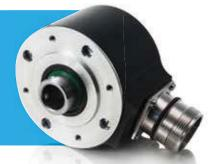
The encoder A58HM is used to measure angular position of the key machine components, industrial robots, comparators, rotary tables, servo drives and to establish an informational link with DCC, NC or Digital Readout Units. The encoder has integrated stator coupling so it can be fixed directly onto object shaft. Mounting adapter - similar to adapter of encoder A58H - is available on request.
