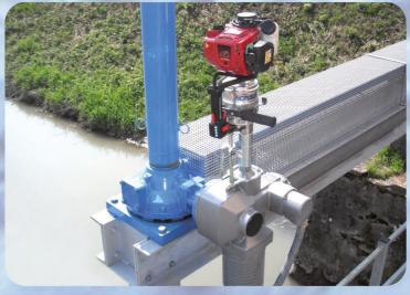
Our actuators are portable devices that have been conceived, designed and certified for handling valves and sluice gates, i.e. mobile control and locking systems placed along rivers, water canals and penstocks, to regulate their flow amount.
