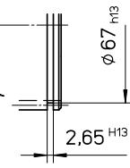
for circlip DIN 471
