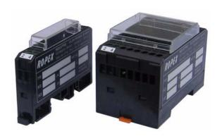
The enclosure of the series resistor can be snapped onto a top hat rail (DIN TS35). The resistor must be installed directly adjacent to the RESISTRON/CIRUS temperature controller. Continuous twisting of the UR measuring wire is essential - including between the series resistor and the controller.
